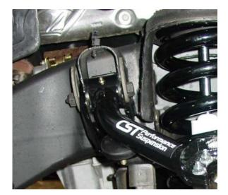
15. GREASE URETHANE BUSHINGS AND INSTALL INTO UCA PIVOTS THEN GREASE STEEL CRUSH SLEEVES AND INSTALL INTO URETHANE BUSHINGS. INSTALL GREASE FITTINGS INTO UCA PIVOTS. INSTALL BALL JOINTS INTO UCA WITH 5/16" x 1 1/2" BOLTS AND HARDWARE, THE BALL JOINT AND THE SPACER SLIPS INTO THE CENTER OF THE TWO PLATES ON THE END OF THE ARM. THE SPACER GOES ON TOP OF THE BALL JOINT.
