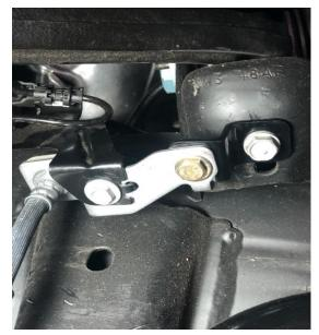
**54.** Route the antilock wire up the spindle and attach it to the spindle and the brake line bracket using the supplied adel clamps and zip ties. Using the factory plastic clips re attach the antilock wires to the frame in the OEM location and connect the wires.Locate the wires so you gain as much slack as possible for the suspension.
