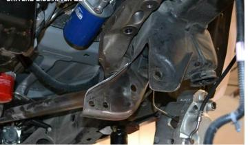
**25.** Cut the passenger side cross member as shown in the picture. It is the front side of the rear lower a-arm mount that gets cut. The cut is horizontal about 3/8" above the top of the two holes. Clean up any sharp edges and paint any bare metal to prevent rust.
