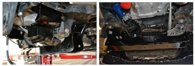
**35.** Install the front sub frame using the stock bolts and Loctite. Do not tighten at this time. (2000 21mm socket, 24mm wrench, 3/4 socket, 3/4 wrench)
