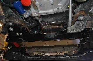
**35.** Install the front sub frame using the stock bolts and Loctite. Do not tighten at this time. (2) 21mm socket, 24mm wrench, 3/4 socket, 3/4 wrench)
