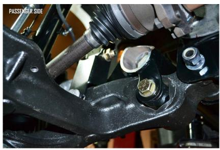
**41.** Reinstall the torsion bars in the truck the way they were removed.
