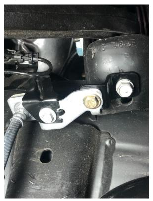
**53.** Route the antilock wire up the spindle and attach it to the bracket using the supplied zip ties. Remove the plastic clip that is pushed into the frame. Run the wire through the hole in the front of the shock bucket so the connector is on the inside of the shock bucket. Attach the antilock wire to the frame using the supplied zip ties. Locate it so you gain as much slack as possible for the suspension.
