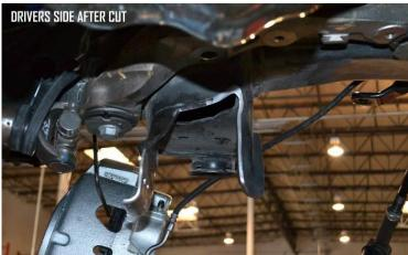
**25.** Cut the passenger side cross member as shown in the picture. It is the front side of the rear lower a-arm mount that gets cut. The cut is horizontal about 3/8" above the top of the two holes. Clean up any sharp edges and paint any bare metal to prevent rust.
