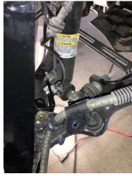
22. ATTACH THE UPPER ABS RELOCATION BRACKET (PART NUMBER 12-116) TO THE REAR OF THE DRIVER SIDE SPINDLE USING THE TOP ¼" HOLE LASER CUT IN THE SPINDLE WITH THE SUPPLIED ¼-20 X 1" BOLT, NUT, AND WASHERS. (SEE PICTURE BELOW) (2000) 7/16" WRENCH, 7/16" SOCKET)
