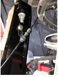
26. ATTACH THE NEW PASSENGER UPPER CONTROL ARM ABS BRACKET (PART NUMBER 12-119) TO THE UPPER CONTROL ARM USING THE OEM BOLT AND THEN CLIP THE ABS WIRE INTO PLACE. BE SURE THE BRACKET IS IN A GOOD POSITION BEFORE TIGHTENING TO ENSURE THAT THE WIRE DOES NOT GET TOO TIGHT WHEN STEERING LEFT TO RIGHT. (SEE PICTURE BELOW) (2)—10MM SOCKET)
