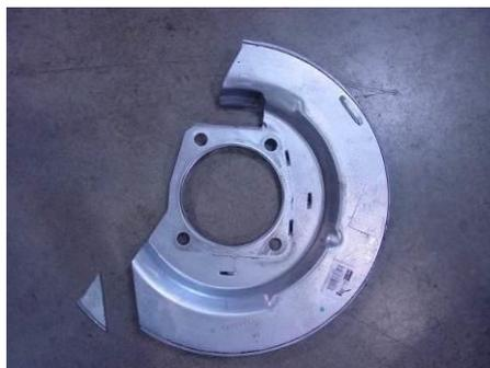
53. Set the new spindle on to the hub and dust shield. Make sure the antilock wire is routed in the correct position through the opening towards the front of the spindle. Bolt the spindle to the hub using the stock bolts and locktite. You must reuse the dust shields. (🔧 21mm socket )
