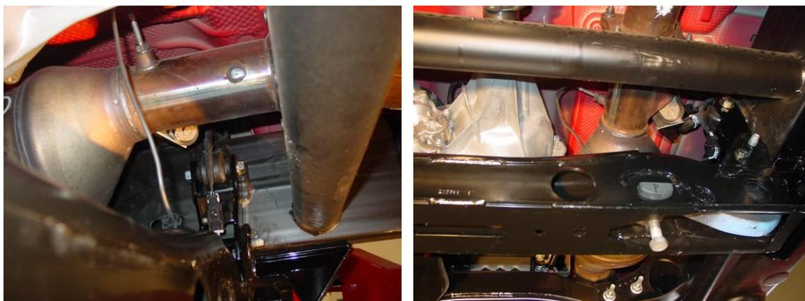
73. Use a large drill bit to put a recess in the torsion key where the adjuster bolt sits against the key. Center it in the key. Use a drill bit between the sizes of 3/4 and 1" and drill it 3/16" deep at the deepest part of the hole. When you are finished it should look like the key in the picture below.
