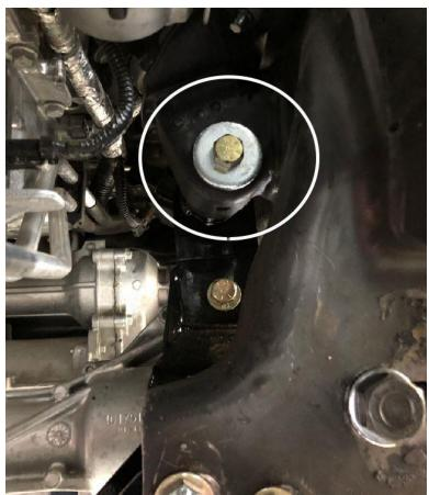
27. Install new CST driver side upper diff drop using the oem bolt (do not tighten at this time).
