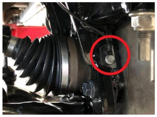
60. Carefully remove the OEM brake line bracket from the brake line on both the driver and passenger side using pliers and a screwdriver to pry it open. See pic below.
