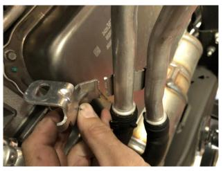
35. Install the provided re-location bracket into the OEM location and then attach the DEF lines to the new bracket using the supplied adel clamp, ¼" bolt, washers, and nut. See picture for reference.
