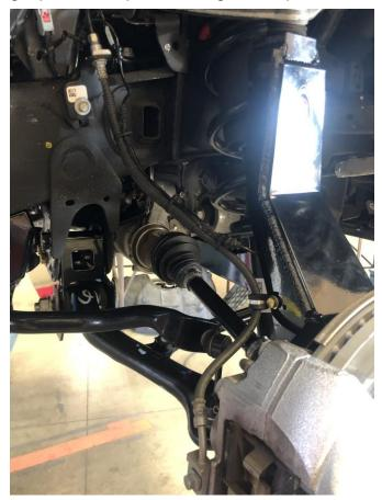
62. On the driver side, remove the ABS wire and speed sensor wire from the OEM clip on the upper arm. Attach driver side oem brake line and front ABS relocation bracket to the rear of the knuckle with the ABS bracket pointed downwards using the supplied ¼" x 1" bolt and supplied adel clamp (7/16 wrench). Clip the ABS wire into new CST bracket. Then zip tie the ABS and speed sensor wire to the brake line in a safe location, so it does not get pinched or pulled too tight. See pic for reference.
