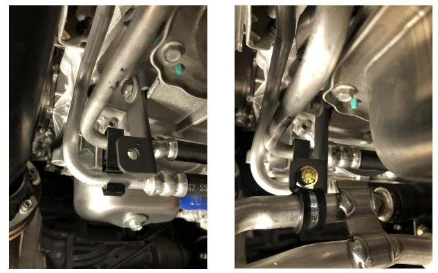
36. Attach the front driveshaft to the front differential using oem bolts. Make sure you line the driveshaft up the same exact way it came off. Use Loctite and tighten all the oem bolts (10mm socket).
