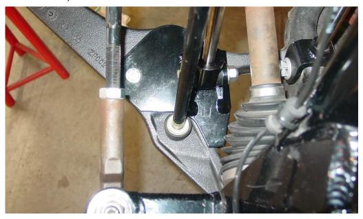
16. Mark the lower hole with the included pattern, and drill it with a 5/16 drill bit. ( mm socket, 5/16 drill bit )
