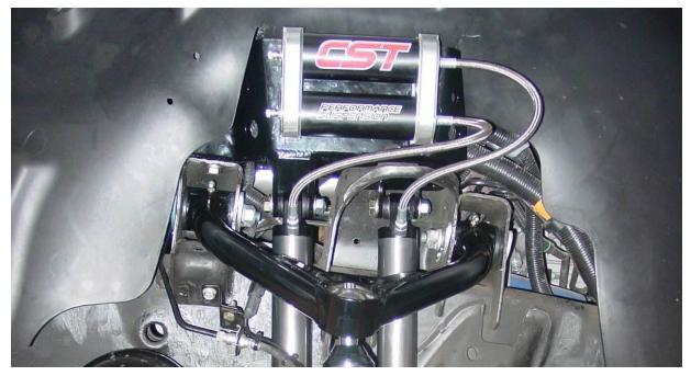
10. Some vehicles may have an air conditioning line that is close to the upper bracket. Make sure the lines are not touching the bracket and have some clearance. Replace the plastic clamp with the supplied adel clamp and ¼" bolt with the bolt side down.
